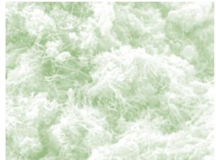
Void completely sealed
